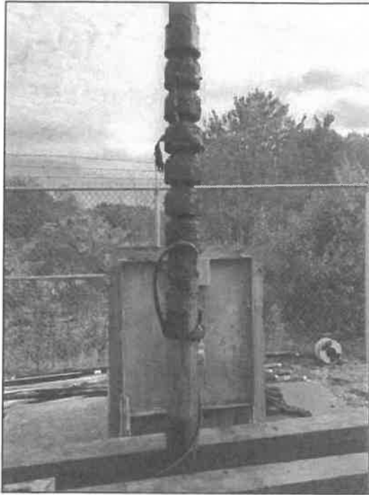
Christensen 6CLC-5 Pump and Centripro 15 HP Motor (left) and clogged intake screen (right) - 9/30/2019
