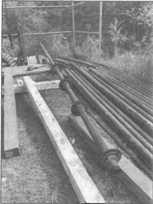
Installation of surge blocks and equipment (left) and initial surge of Bedrock Well #2 (right) - 10/1/2019
