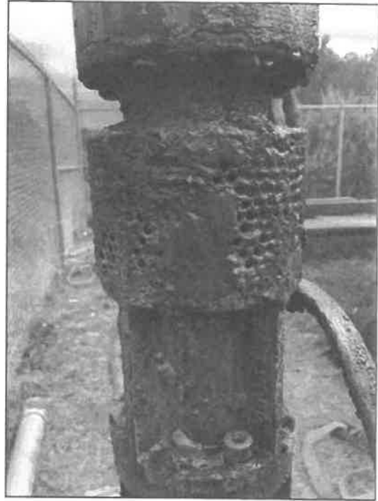
Christensen 6CLC-5 Pump and Centripro 15 HP Motor (left) and clogged intake screen (right) - 9/30/2019
