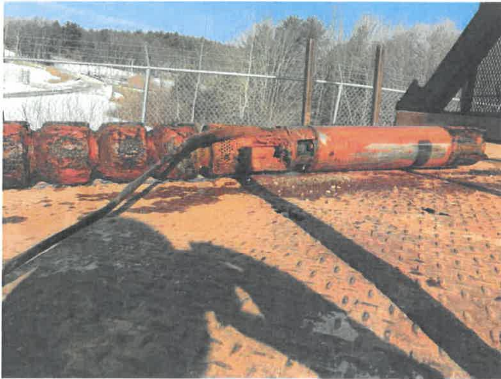
Christensen 6CLC-5 Pump and Centripro 15 HP Motor (left) and clogged intake screen - 1/12/2022
